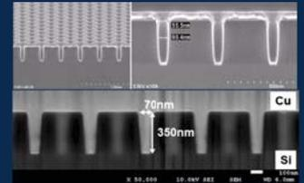
Defect free Cu filling was confirmed[1]
