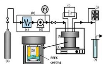
(a)CO<sub>2</sub> gas tank, (b)CO<sub>2</sub> liquidization unit, (c)liquidization unit, (d)high pressure pump, (e)thermal bath, (f)reaction cell (SUS316L) with PEEK coating inside, (g)substrate, (h)cross stirrer, (i)power supply, (j)back pressure regulator, (k)trap
