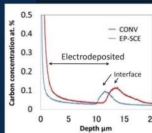
Theoretical film thickness, about 12 μm
