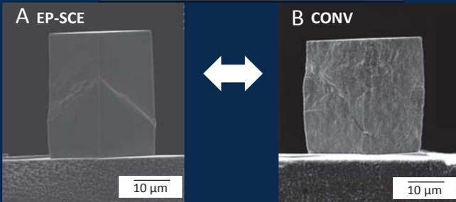
• Shear band was observed for EP-SCE
